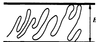
Figure 4. Tilted chain. By tilting, the chain increases the arc-length it uses in going between the plates. This lowers the confinement free energy.
